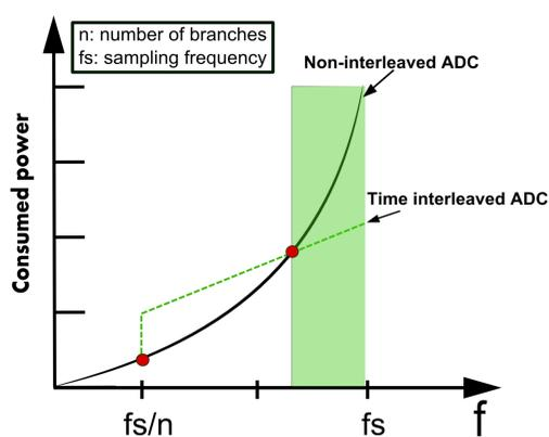
Fig. 1. Time-Interleaving Concept
