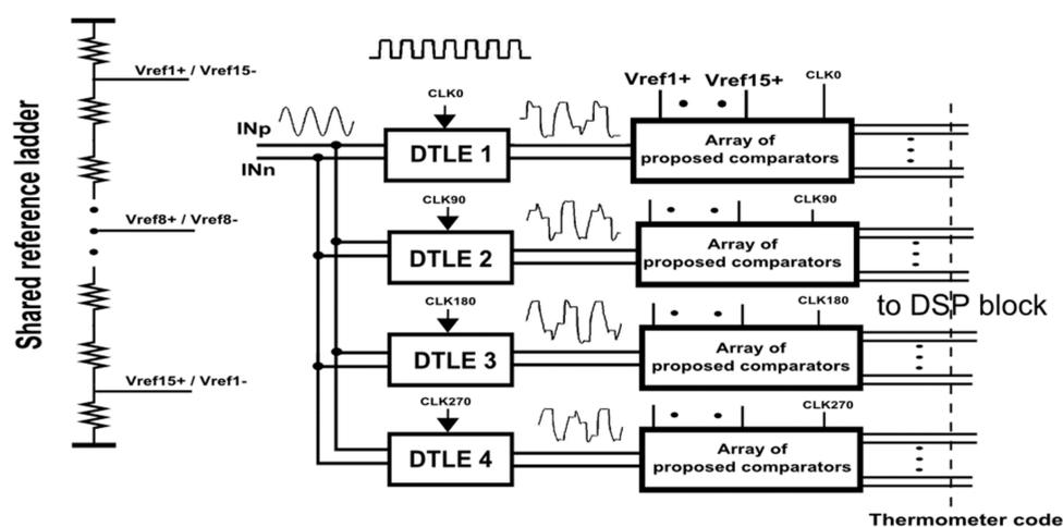
Fig. 3. Architecture of ADC-based Equalizer
